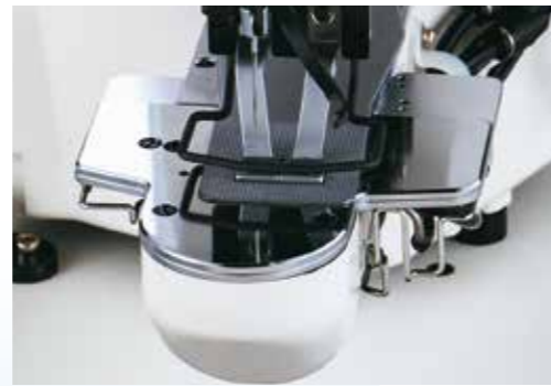
Bird's nest preventing /Shorter-thread remaining functions
