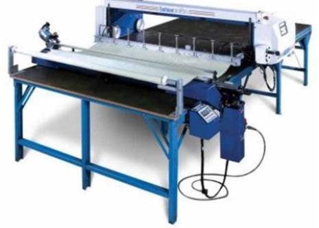
The Blue Jay is available as a stand-alone end cutting unit or with an optional Pull-Off for even faster cutting production and improved accuracy. The system requires only one operator to spread and cut material with the simple press of a button.
