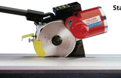
Eastman's Falcon IV's superior balance and specially designed Falcon track allows the knife to glide effortlessly across the guide track for perfectly straight line end cuts.
