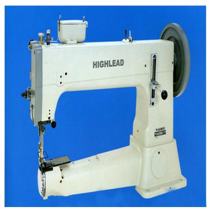
Max Sewing Speed 800 r.p.m. Stitch length 0-11 mm Needle bar stroke 56 mm Thread take-up lever stroke 96 mm By hand/knee 13 / 20 mm Pressure foot lift Bed size in dia. 81 mm 400 mm Bed length DY x 3 26# Needle size Shuttle hook KSP-204N
