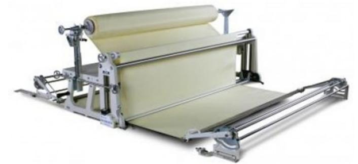
Eastman's top-of-the-line manual spreader, the Pacemaker, can be utilized efficiently and with ease for face-up and face-to-face spreading.
