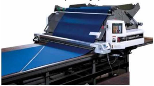
The Saber C-Series computerized, cradle feed machine is a robust yet smooth operating material spreading sysetm with models suitable for up to 2,200 lb. rolls.
