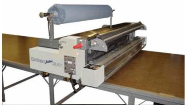
The Eastman Saber Select™ positive feed system is designed for spreading rolls of material with weights up to 500 or 800 lbs. (227/363 kg).
