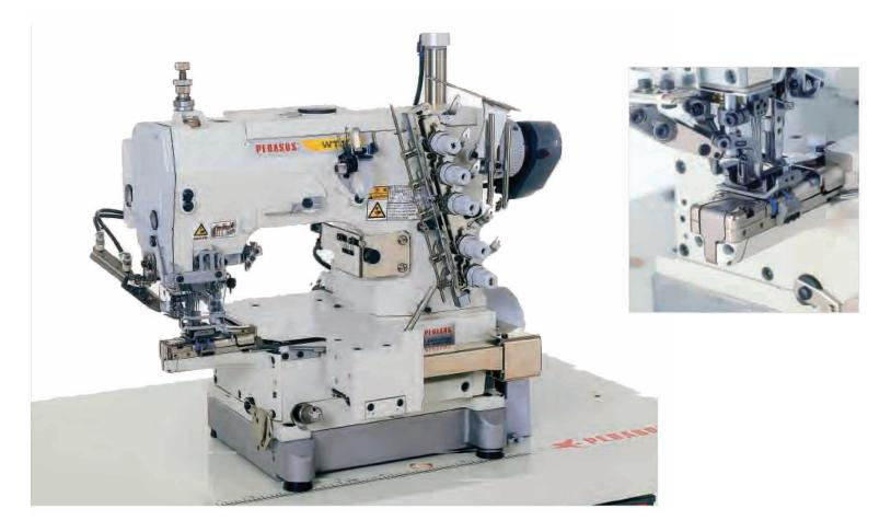
3-needle, variable top feed, interlock stitch mahine with extremely small-sized cylinder bed for hemming.
