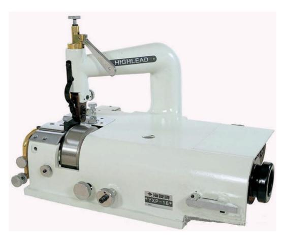
A high quality skiving or material scraping machine that is used to skive all kinds of leather products, synthetic leather and rubber articles. It comes equipped with an automatic chip cleaner and knife sharpening clutch. Skiving width is adjustable from 15 mm to 50 mm.
